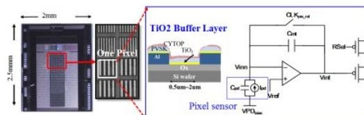
Figure 2. The photo of CIS chip and read-out circuit
