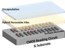
Figure 3. Illustration of perovskite film vertically integrated on the top of signal read-out circuit
