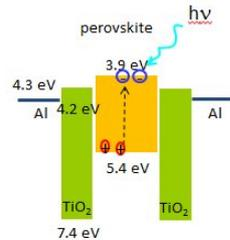
Figure 8. The energy diagram of the planar-electrode perovskite photodetector
