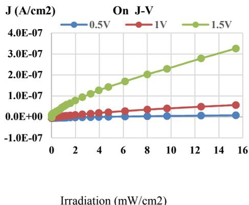
Figure 9 Current density vs. Irradiation curve of perovskite CMOS image sensor
