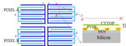
Figure 1. Structure of planar-electrode perovskite photodetector on dummy chip
